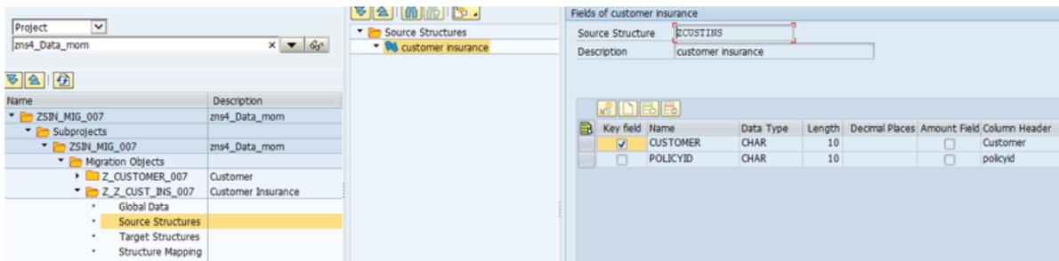
8. Above structure would create a template for migration cockpit. Some fields can be made mandatory or disabled by making some changes in customer view of this structure. Right click on structure name and select 'display view'. Below view is Customer view.
