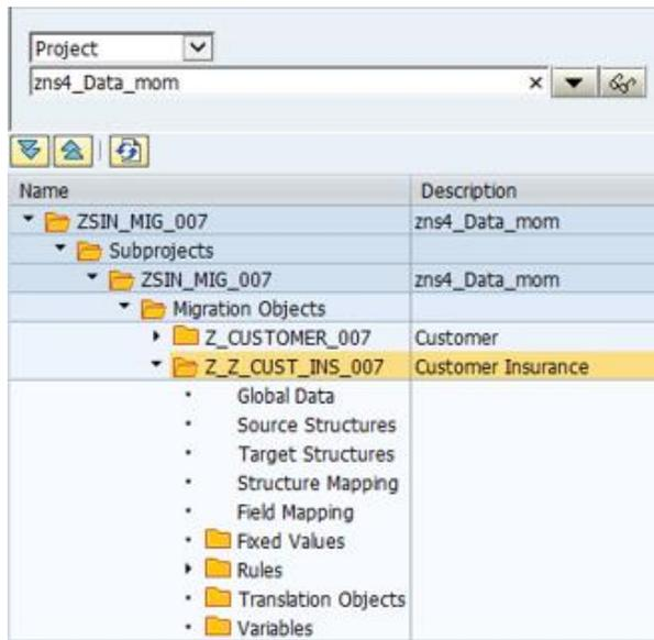
7. Double click on source structure, it will open a new window on left. Define new structure and its fields as follows.
